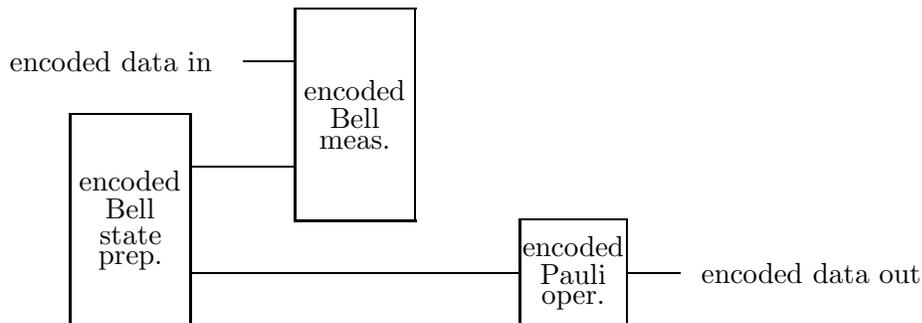
First the encoded Bell state  $\bigotimes_a |\bar{\phi}_a^+\rangle_{BC}$  is prepared and verified, then encoded Bell measurement is performed on block  $B$  and the incoming data block  $A$ , and finally an encoded Pauli operator is applied to complete the teleportation of the incoming encoded state.
