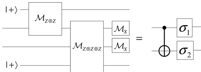
Here  $\mathcal{M}_\sigma$  represents measurement of the Pauli operator  $\sigma$ ,  $|+\rangle$  is the eigenstate of  $X$  with eigenvalue  $+1$ , and  $\sigma_1, \sigma_2$  on the right-hand side of the equation are single-qubit Pauli operators that depend on the outcomes of the four measurements in the circuit on the left-hand side. What are  $\sigma_1$  and  $\sigma_2$ ? **Hint:** Check that Pauli operators propagate through the circuit as they do through a CNOT gate:
