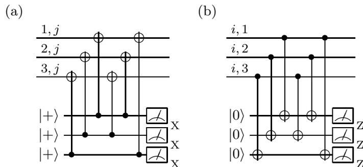
E.g., for  $j = 1$ , the procedure (a) measures  $X_1X_4$ ,  $X_4X_7$ , and  $X_1X_7$ , and for  $i = 1$ , the procedure (b) measures  $Z_1Z_2$ ,  $Z_2Z_3$ , and  $Z_1Z_3$ . Though  $X_1X_7$  is not independent of the other two observables in the first column, this third redundant measurement is needed to ensure fault tolerance. Similarly, in (b) the third measurement in each row ensures fault tolerance.
