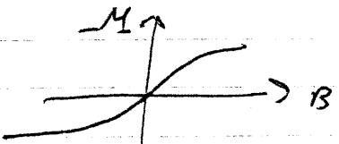
Now  $B$  is the magnetic field seen by a spin - which depends on magnetization as well as applied field
